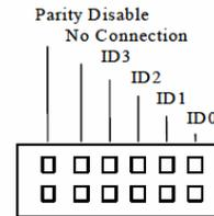
Figure 3-3: Jumper positions
